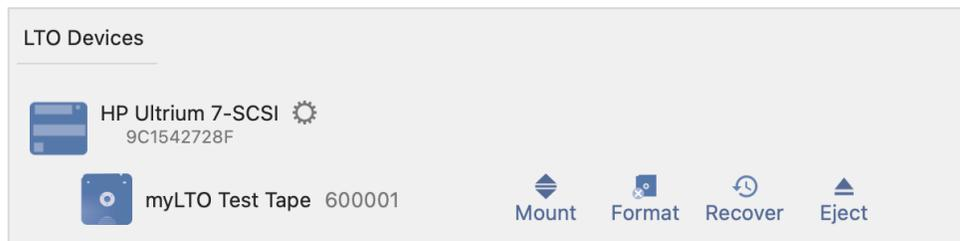
If you've enabled the **Eject on Dismount** option, the tape should be expelled from the LTO drive once the unmounting has completed.
