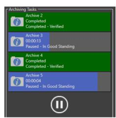
CAUTION! Do not quit the application or force Eject the tape while a backup session is being processed. Doing so may create incomplete files or even damage your LTO tape. Click the 'Pause' or 'Cancel ALL' button at the bottom of the Archiving Tasks list before un-mounting (or ejecting) a tape.
